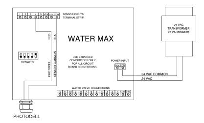
TRANSFORMER NOTE: Use machine tool variety, 40 VA minimum is recommended. If a larger transformer is used, adjust the fuse protection accordingly.
